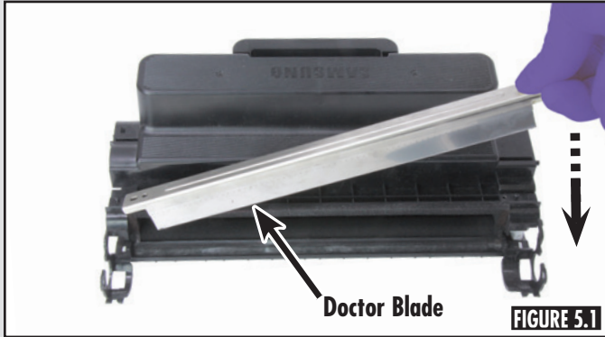
Align the doctor blade as shown and place onto toner hopper. (Figure 5.1)
